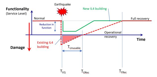
Figure 8.3: The difference in functional impacts of earthquakes on new and existing IL4 buildings
