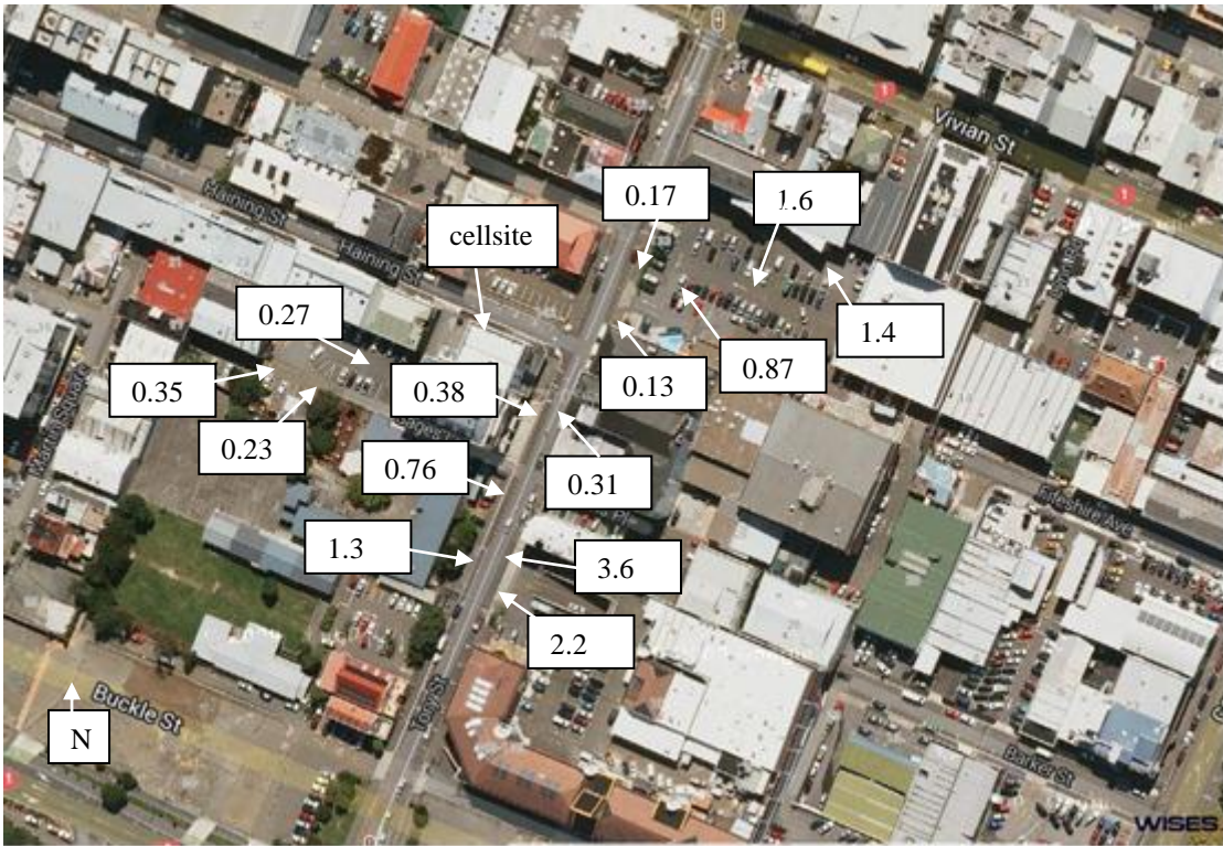
Figure 5 Tory Road Relocate cellsite layout showing measured power flux density ( \mu\text{W}/\text{cm}^2 )
