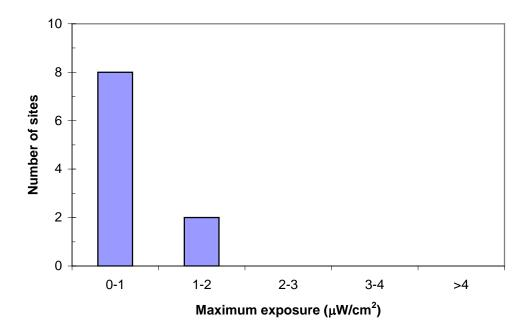
At most of the sites tested, the maximum exposure was less than 1 microwatt per square centimetre ( $\mu W/cm^2$ ). Two sites had a maximum exposure greater than 1  $\mu W/cm^2$ ; but were below 2  $\mu W/cm^2$  and both had other transmitters nearby.
