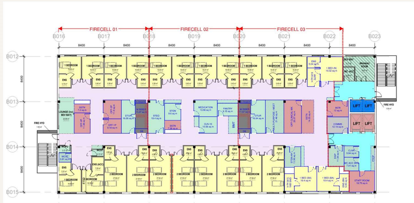
Alternative Test-to-fit layout using central riser strategy, 4 fire compartmentation, and updated HPU
